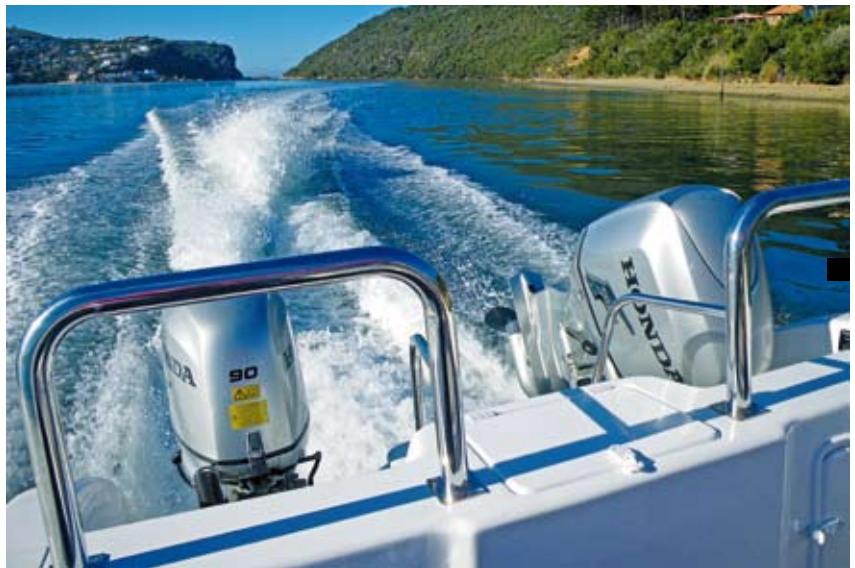
Interestingly, skipper Derik Meintjies shows that the Sailfish 200 is more than capable of planing with just one motor in the water.
