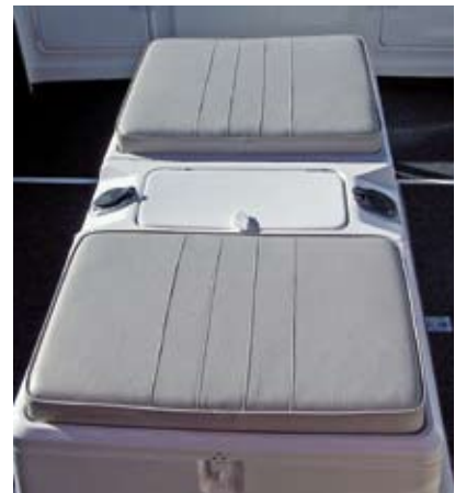
A storage hatch situated in the middle of the deck not only provides adequate seating, but also sufficient storage.
