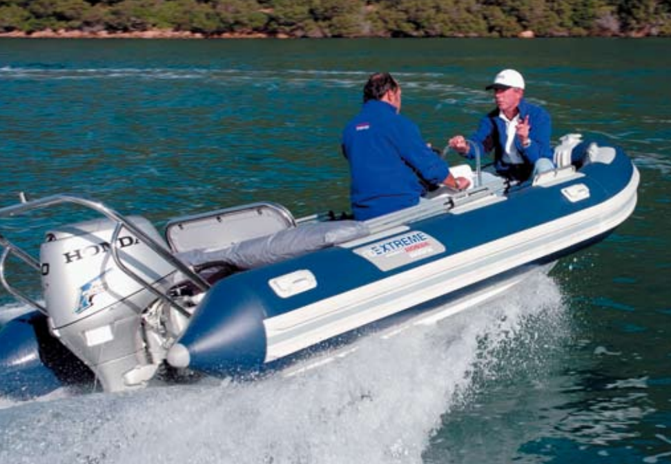
Pontoons are made of German Valmex and all seams are thermo-bonded.
